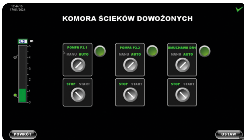
FIGURE 23. Settings of the technological process of the treatment plant, with the possibility to change the operating modes
